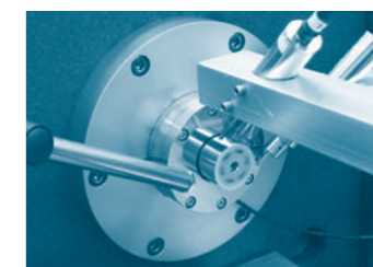
State of measurement (Non-contact type electrostatic displacement gauge is used.)
